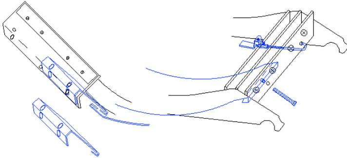
Use bottom holes for Cover Plate installation using either bolt or Cover Plate Handle
